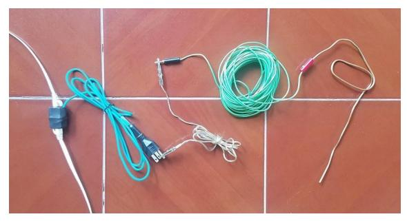
To do this, you will need two <u>Cat-7 Shielded Ethernet cables</u>, an <u>Ethernet Ground Adapter</u>, <u>Gator-to-Gator connector</u>, <u>50' extension cord</u> and an 18" copper stake that you can get <u>here</u> or at your local hardware store.
