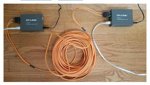
In the picture above, your modem/router is connected to the Ethernet cable coming from the right. This cable connects to the first fiber converter and the data is converted to light to be transmitted via the fiber optic cable to the second converter at left. From the second fiber converter, you will run an Ethernet cable toward your laptop. However, you want to ground that cable to the outside before it gets to your computer, as seen in the following picture:
