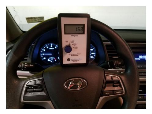
The magnetic field shown above is from a 2017 Hyundai Elantra with the engine running. The field drops to about 0.3 mG at the driver and passenger seats, which is quite low.
