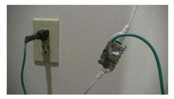
An Ethernet Ground Adapter will reduce much of the EMI flowing to your computer.
