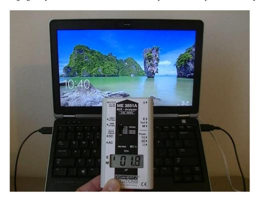
This electric field measurement was taken just a couple minutes later once the proper setup was in place. The only difference is there is now almost no EMI transmitted by the Ethernet cable. Electric field readings below 3 V/m are much healthier for any extended use of your computer.
