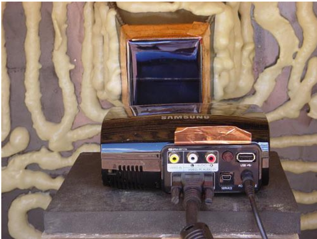
The projector is in a shielded box and sends the images through an inverted lens.
