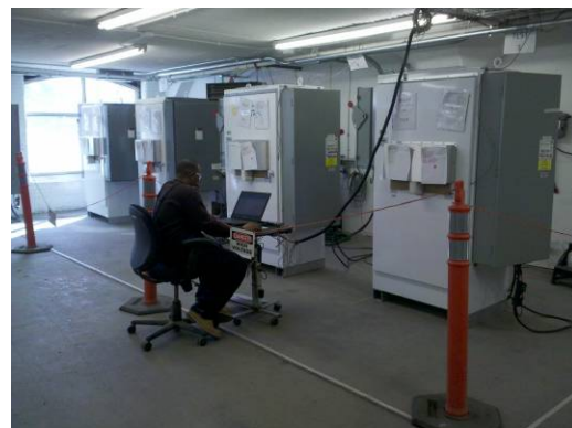
8 Hour HASS Burn-in Test and Final Verification
