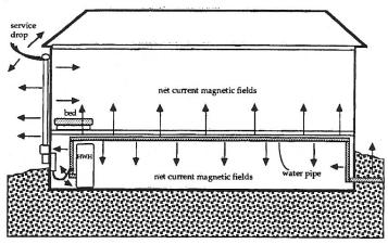
**Net current - Splitting between electric service & water system grounding.** Net current path as neutral return current splits at service point due to required grounding to water system at other end of house. Indoor pipe has current; service drop has same net current due to a deficit of the neutral.
