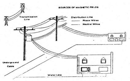
**Net current** – Current in electric supply is shared with water service lines between buildings. Part of the return, "spent" current travels between buildings through conducting water pipes. Electric distribution lines are not balanced because the neutral wires no longer have equal (and cancelling-effect) current to "hot" phase wires – and comparatively generate higher magnetic fields. The water pipes also become emitters of magnetic fields.
