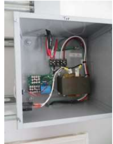
Figure 24 DNA Line Filter.
