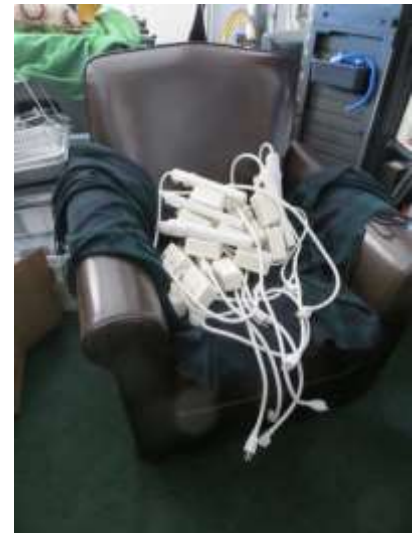
Figure 23 Removed parallel filters.
